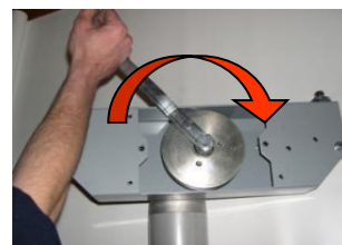
8 Now the motor shaft and reduction unit are released from the pulley and we can go on with the covering manual handling.
