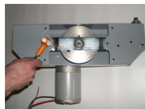
3 Using the same Allen key, loosen the 2 screws of the motor shaft reinforcement bracket.
