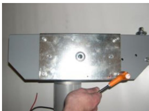
1 By using a 6 mm Allen key, loosen the 4 screws of the protection cover
