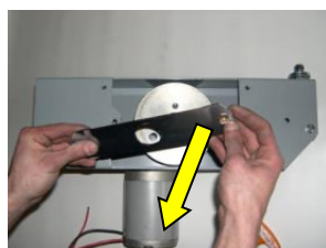
5 Extract the bracket from the bearing.
