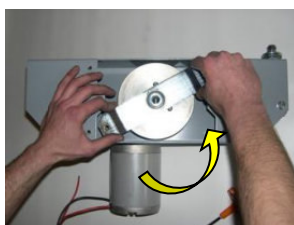
4 Rotate the bracket as in the picture.
