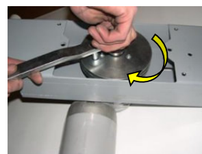
7 Tighten up the handle screw to the end, using if necessary a wrench for hexagonal screws.
