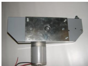
1 By using a 6 mm Allen key, loosen the 4 screws of the protection cover
