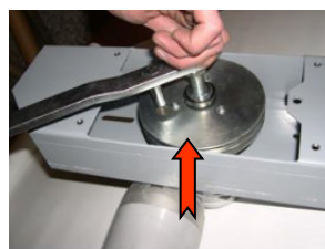
6 Tighten up the emergency handle in the centre of the shaft, paying attention to introduce the round pin into its proper seat.
